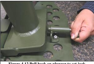
Figure 4.12 Pull back on plunger to set jack.
