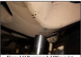
Figure 4.14 Recommended lifting point.
