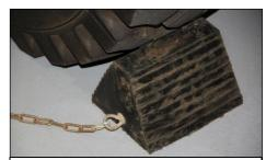
Figure 4.1 Wheel chocks are not supplied in 88M-MPBMI Jack Kit.
