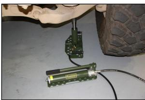
Figure 4.13 Position Jack in line with vehicle axle. (Parallel)
